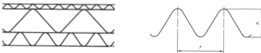
Figure 7.2-1: Triple-wall corrugated fiberboard (left) and Flute dimension (right)
